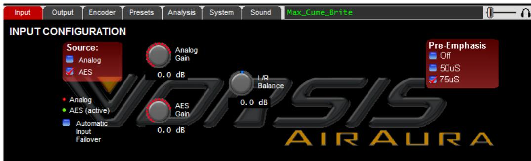
While still in the Input menu and observing the Input meters adjust the Input Gain control (AES or Analog as required) until the input meters are just peaking around -12dBFS with normal program levels being applied.
