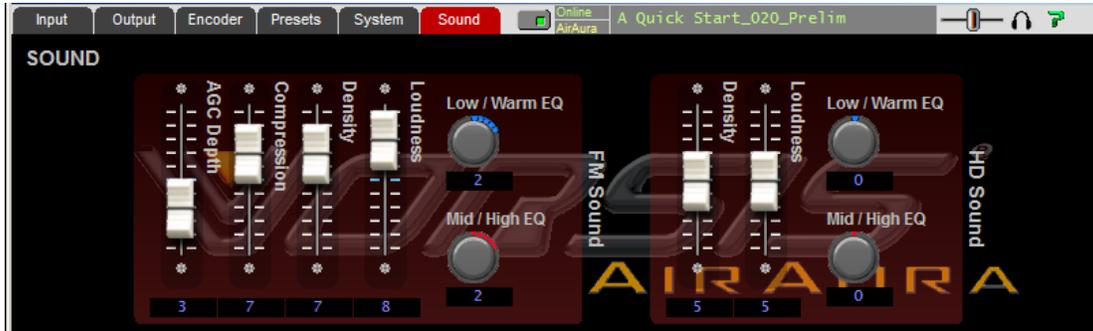
There are two sections to the Sound screen. The left side contains the controls that modify the sound of the FM signal path while the right side hosts the controls for adjusting the sound of the HD signal path. Note that the FM and HD signal paths share a common five-band AGC structure in order to maintain a consistent spectral texture as an HD receiver blends from analog over to HD.
