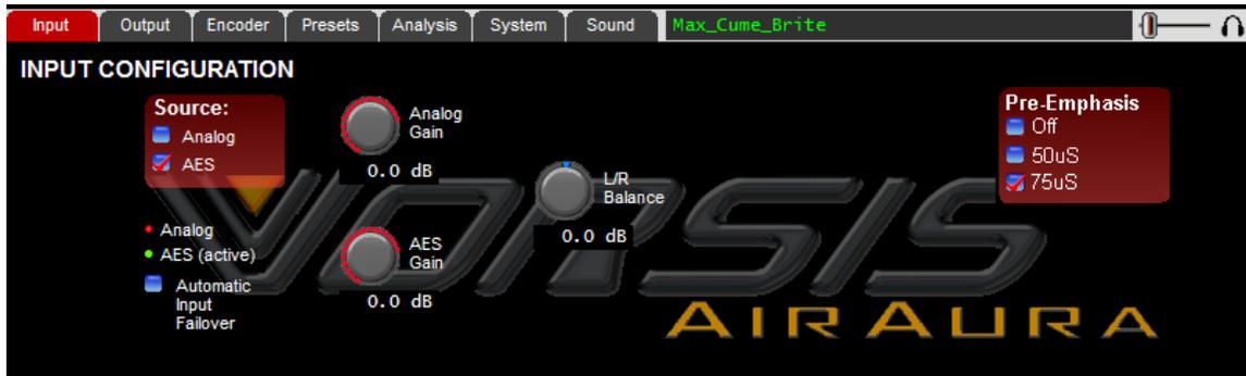
The Input screen contains controls for the Input Audio Source, Automatic Failover Enable, Analog and AES/EBU input gain controls, input L/R gain balance, Phase Rotator In/Out, and Pre-Emphasis selections.
