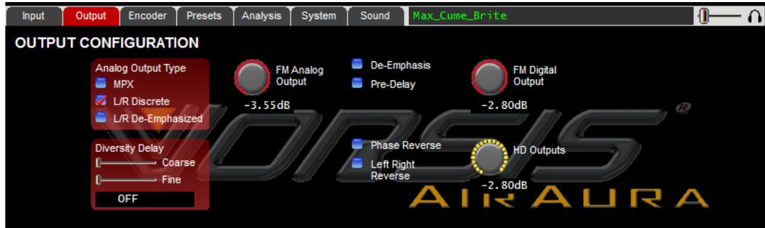
Next adjust the FM Analog Output control to set the correct Left and Right output level.
