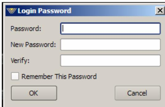
Remote login is for password restricting GUI access to an AirAura processor over the Ethernet connection. When a GUI TCP connection session is initiated, AirAura accepts the connection and then asks the remote GUI for a password.
