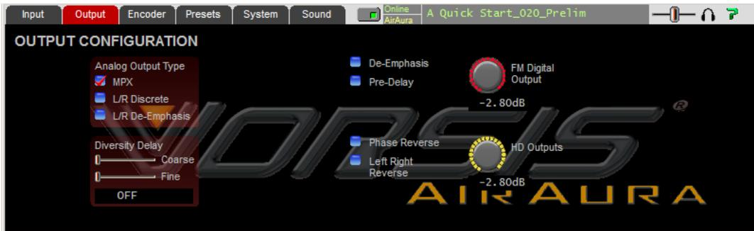
The Output screen contains controls for the Analog Output Type, FM Diversity Delay, FM Digital Output level and the HD Output levels.
