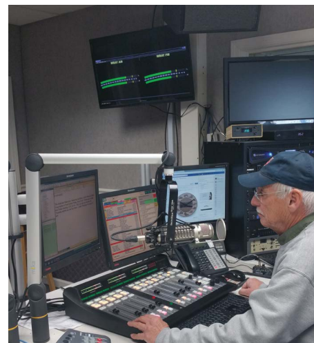
WRAY(FM)'s studio also features the WheatNet-IP-metering app, seen on a large monitor in-studio, monitoring the output of the final blade in the air-chain. Dave Kunkle assesses the situation.
