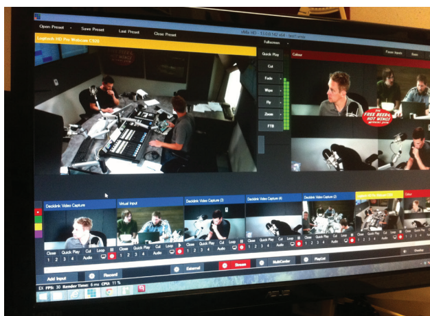
vMix software handles video switching, graphics and encoding
