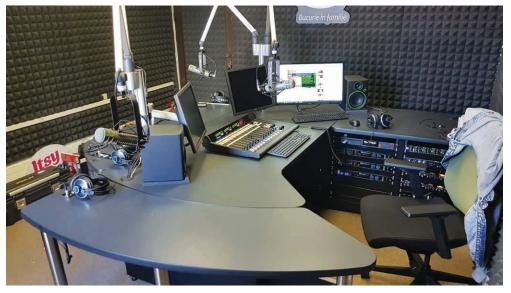
that make up a WheatNet-IP audio network. We needed rack space below the counters for the I/O units and we required a free-form countertop that was rugged and fit the flow of our busy format. Itsy Bitsy broadcasts kids programming out to more than 60 percent of the country.
