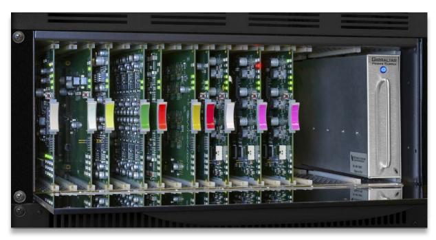
The core switch can connect to 48 I/O Gibraltar Network frames, each capable of over 512 audio I/O paths. Because the frame's audio cards are front loading, service can be performed in real time. A selection of cards provides translation from analog, digital, SDI, and MADI inputs or outputs. Naturally, redundant cards can stand ready in each frame for those applications where failure is simply not an option.
